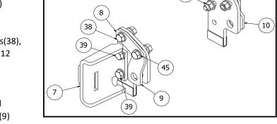
Attach using two M12-1.75 X 45 Bolts(38), one M12-1.75 X 35 Bolt(39), three M12 Washers(45), and three M12-1.75 Nuts(50). Tighten the bolts and nuts
