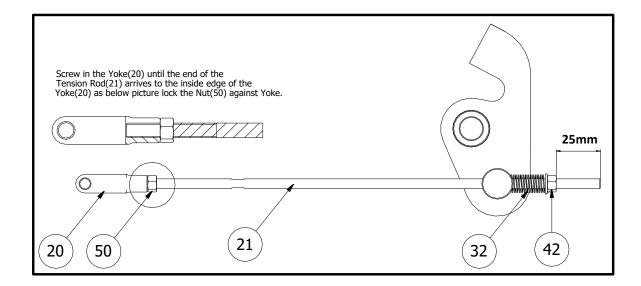
Note: Operator should check and set the clearance(30 mm) periodically during using the mower.
